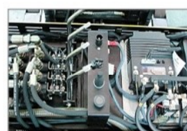
Double controllers with CANbus communication to oil tube and wire
